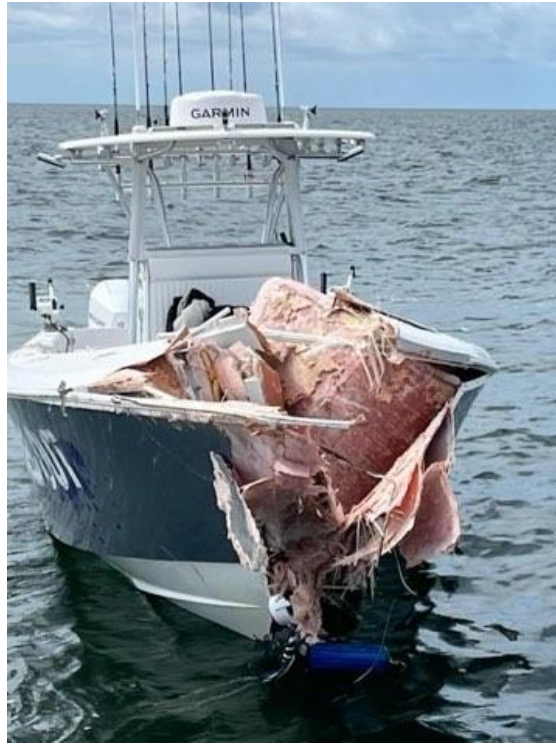
Figure 4. LINEDOUT bow damage from impact, Taken March 12, 2024. Source US Coast Guard.
